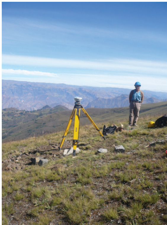
Figure 12.3. A GPS 5800 II measuring the A006 C-Order benchmark.
